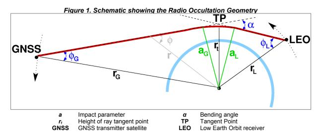
From the 'profile' of **bending angle** as a function of **impact parameter**, a profile of **refractivity** as a function of **geometric height** can be obtained, and thence profiles of **pressure**, **temperature** and **humidity** with **geopotential height**. It is out of the scope of this document to describe the details of these steps, but see for instance [RD.9] for a description of the RO technique and the derivation of geophysical quantities.
